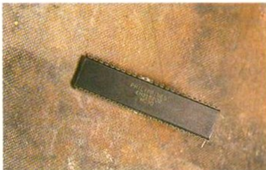
An all too common sight is a pin out of line. It's impossible to insert a chip in this condition – don't even try it.
